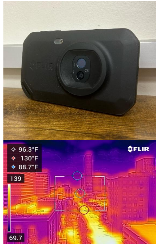
Figure 4. FLIR C-5 camera used in this pilot program and an example FLIR image from an urban canyon in Austin, Texas.
