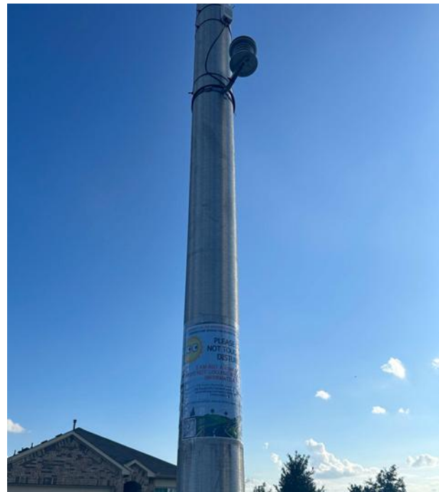
Figure 3. HOBO Sensor and poster mounted on light poles in the Treated Site.
