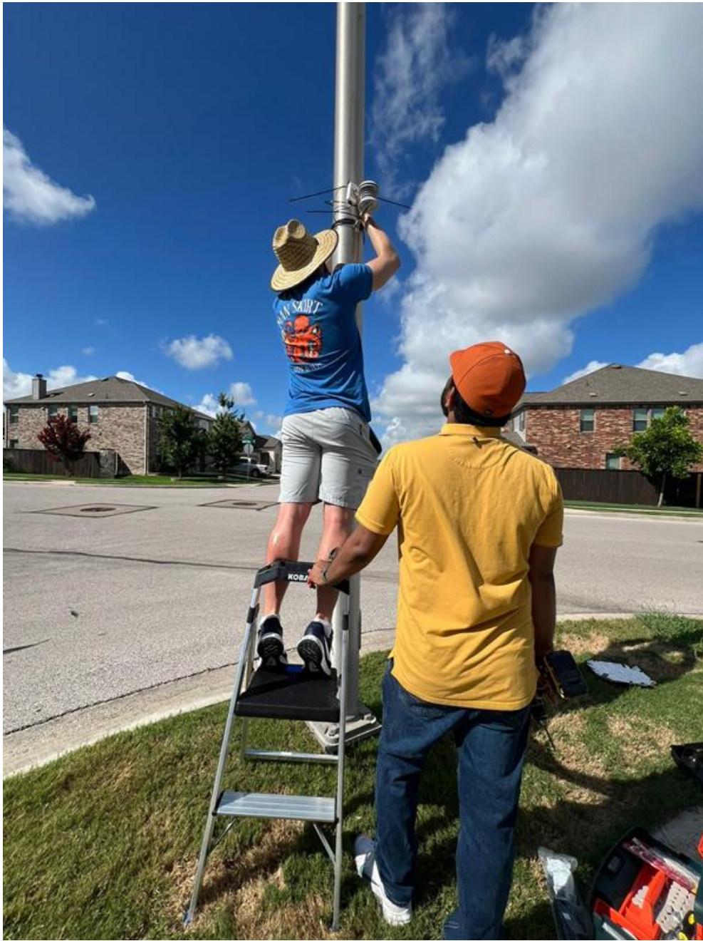
Figure 3A Researchers installing HOBOT air temperature sensors before the treatment was applied
